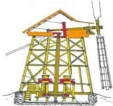
**Fig. 3. Windmill – section**
