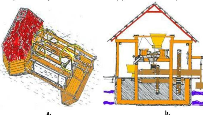
**Fig. 1. Floating - Mill: a - view, b - section**
