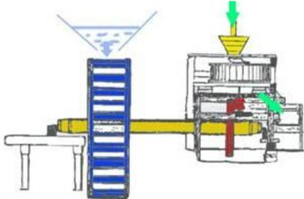
**Fig. 5.** Die with vertical well (principle)
